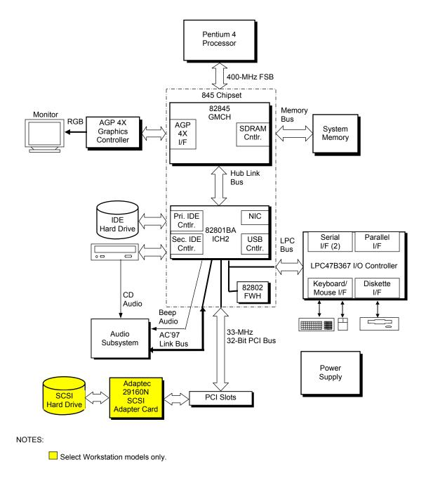
Figure 2–9. System Architecture, Block diagram
